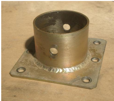
Fig. 1: Flange without strengthening ribs
